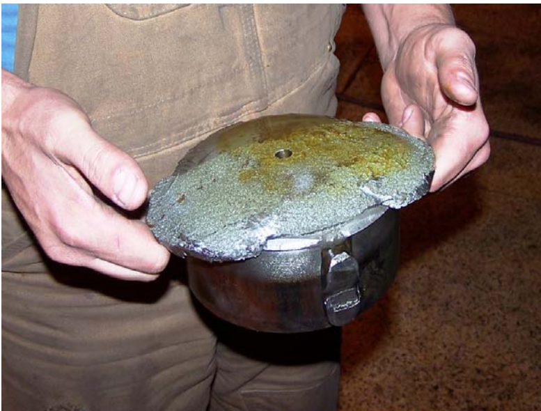
Photo A-5. Broken Inside End of the Link Pin, John Day
