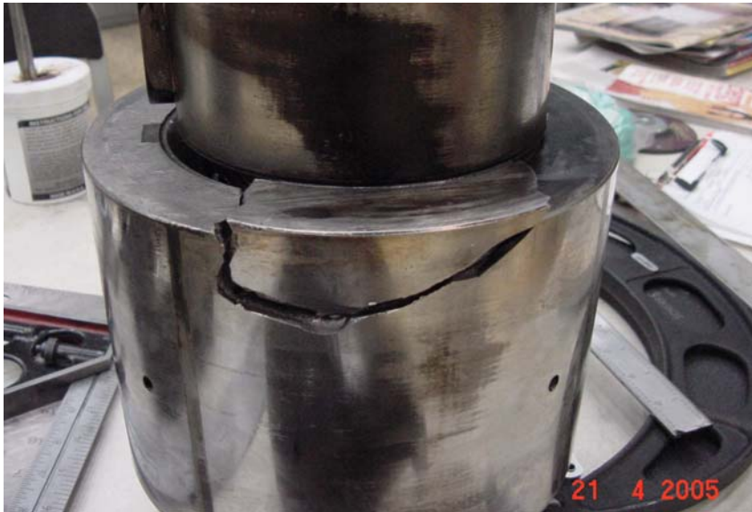
Photo A-3. Lower Pin After Removal from Runner Hub, Lower Monumental Unit 1
