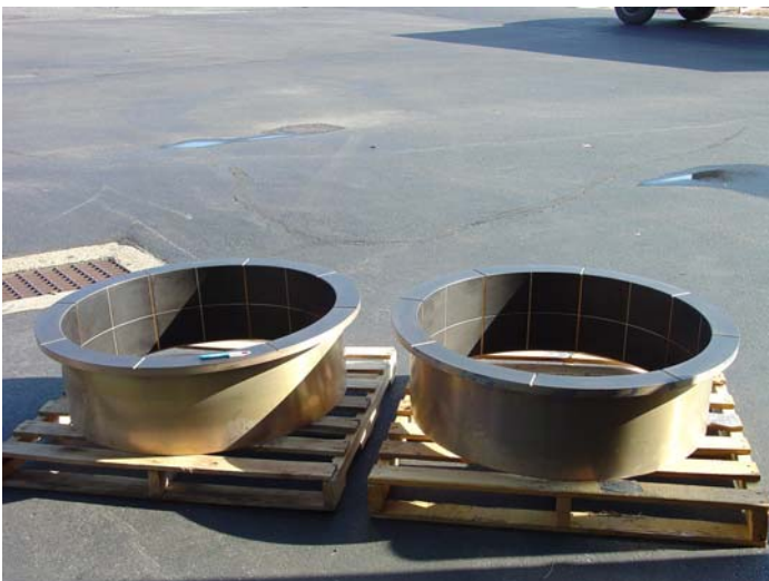
Photo J-2. Coated Outer Blade Bushing (~36 inches in diameter)
